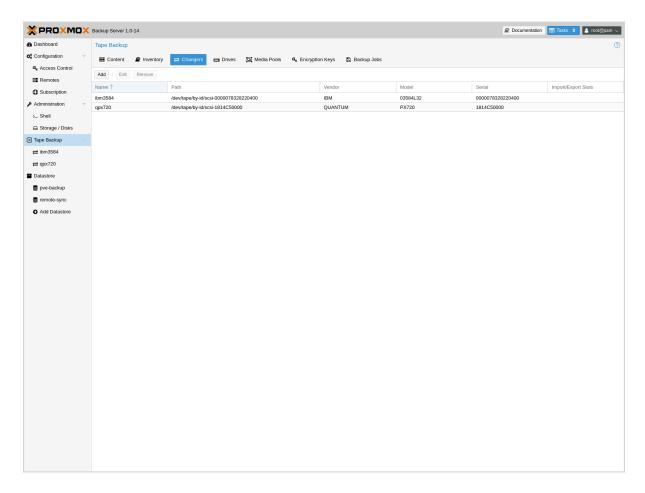
Tape changers (robots) are part of a Tape Library. They contain a number of slots to hold tape cartridges, a barcode reader to identify tape cartridges and an automated method for loading tapes.
