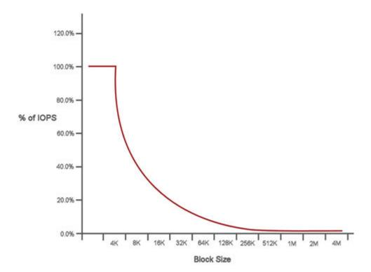
As an example, if block sizes are 4k, and bandwidth is 4000 KBps, the IOPS are 1000. If block sizes increase to 8k, bandwidth increases to 5000 KBps, and IOPS decrease to 625. By taking block size into account, the system ensures that lower priority workloads that use higher block sizes, such as backups and hypervisor activities, do not take too much of the performance needed by higher priority traffic using smaller block sizes.
